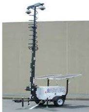
Portable C-WATCH System Telescopic Mast & Generator
